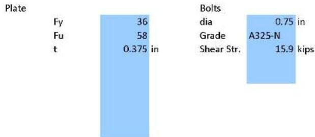
**8 Flexural Rupture of the plate**
